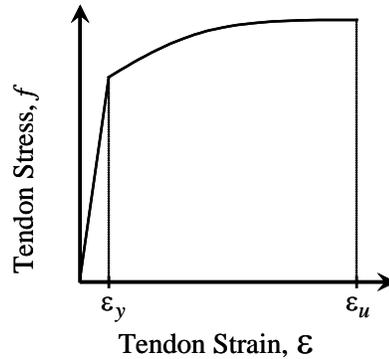
Figure 5 Tendon 270Ksi Strand Stress-Strain Curve
