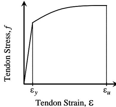
Figure 4 Tendon 250Ksi Strand Stress-Strain Curve
