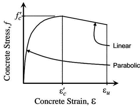
Figure 6 Simple Concrete Parametric Stress-Strain Curve
