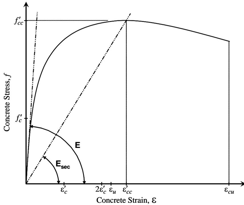
Figure 8 Mander Confined Concrete Stress-Strain Curve
