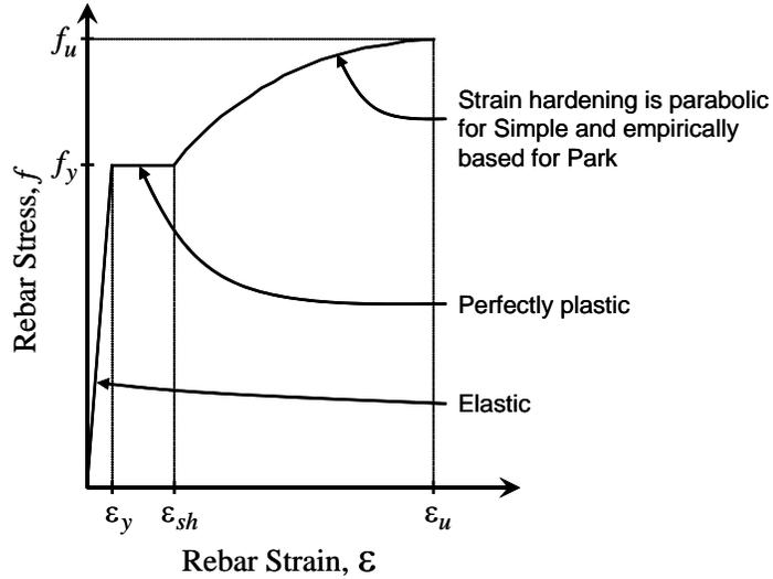
Figure 2 Rebar Parametric Stress-Strain Curve
