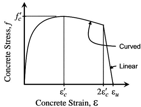
Figure 7 Mander Unconfined Concrete Stress-Strain Curve
