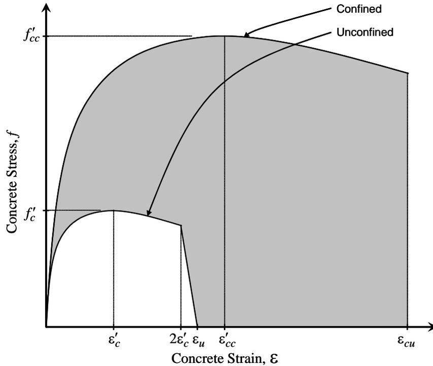
Figure 9 Mander Confined and Unconfined Stress-Strain Curves
