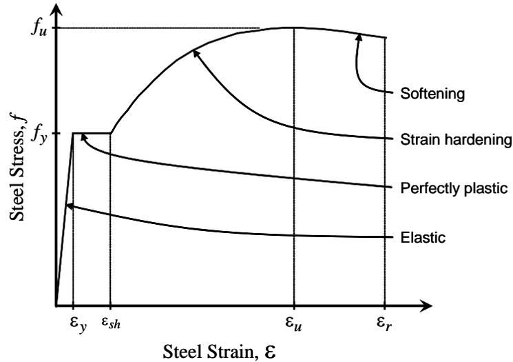
Figure 3 Simple Structural Steel Parametric Stress-Strain Curve
